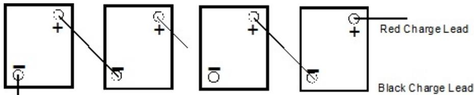
When batteries are connected in series, the voltage is additive, and the amp hour rating remains the same. Example: four 100 amp hour, 12 volt batteries would equal 48 volts, and 100 amp hours of capacity.
