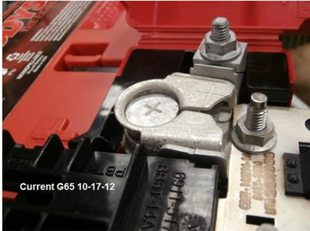
The combination of the step on the battery cover and the terminal distribution block on the positive cable prevents the positive connector from being adequately torqued – the connector does not sit far enough down on the positive post of the battery to facilitate a secure connection.
