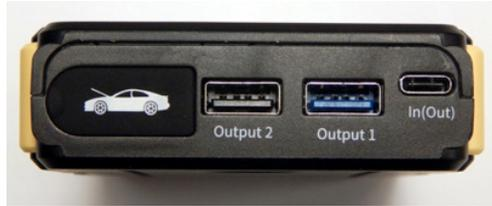
Before using the E-Power, make sure that it is fully charged. This unit is charged through the USB-C port. A 12" long charging cord is included. One end with USB-C to plug into the E-Power (to the port labeled In(Out)), and the other end is USB-A that you can plug into a cell phone charger port, a USB port in a vehicle, or a computer USB port.
